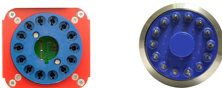
Fig. 5.1: The socket cavity of Hawkeye is designed to fit into the PMT base socket. Check the correct mounting of Hawkeye on the PMT itself
