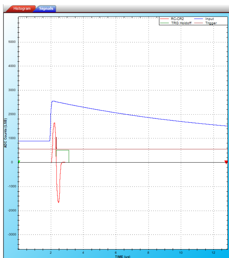
Fig. 6.12: Signal Inspector view showing the Input and the RC-CR2 traces in case of faster signals
